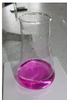
phenolphthalein Alkali colour
