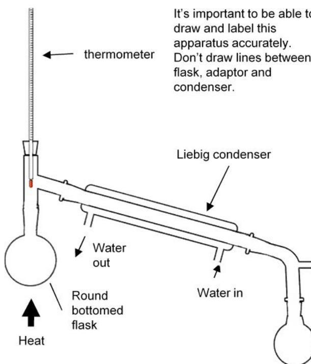
It's important to be able to draw and label this apparatus accurately. Don't draw lines between flask, adaptor and condenser.
