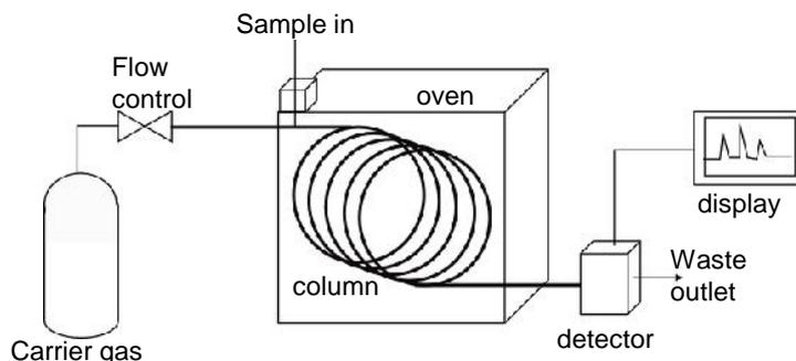
Most commonly a mass spectrometer is combined with GC to generate a mass spectra which can be analysed or compared with a spectral database by computer for positive identification of each component in the mixture.
