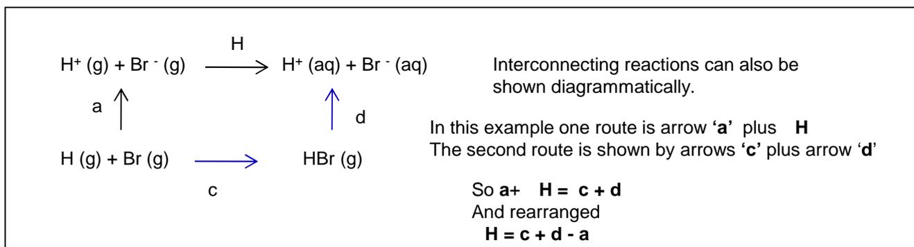
Often Hess's law cycles are used to measure the enthalpy change for a reaction that cannot be measured directly by experiments. Instead alternative reactions are carried out that can be measured experimentally.
