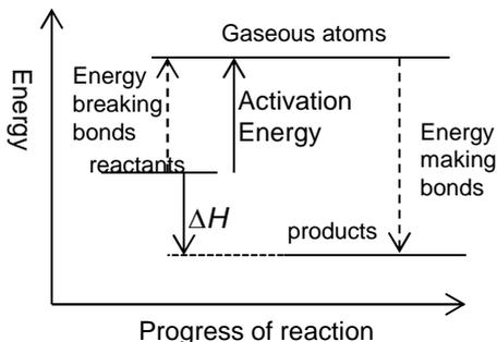
Bond breaking absorbs energy and bond making releases energy
