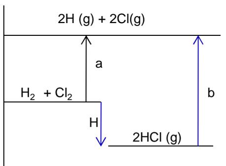
On an energy level diagram the directions of the arrows can show the different routes a reaction can proceed by.
