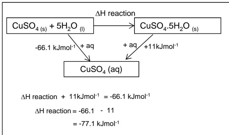
This Hess's law is used to work out the enthalpy change to form a hydrated salt from an anhydrous salt.
