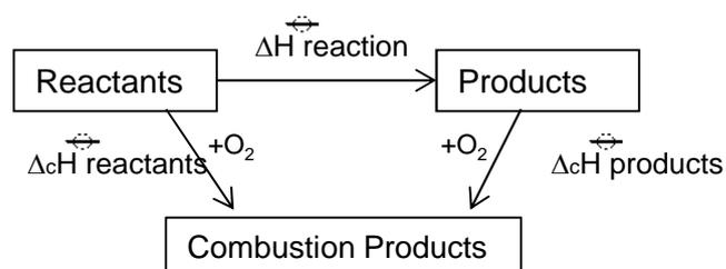
**Example 8.** Use the following combustion data to calculate the enthalpy of reaction
