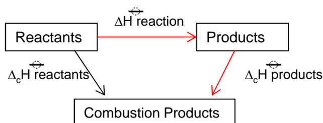
$$U_c H \text{ reaction} = U_c H \text{ reactants} - U_c H \text{ products}$$
