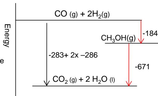
Note: unlike enthalpies of formation, elements do have an enthalpy of combustion value. Burning hydrogen in oxygen is a very exothermic reaction!
