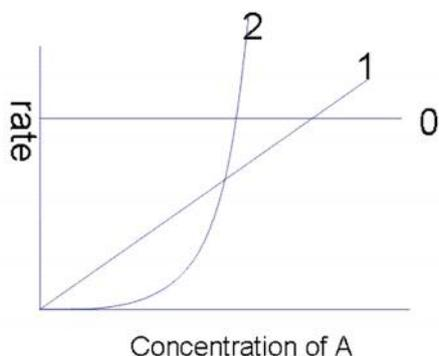
For zero order: the concentration of A has no effect on the rate of reaction  $r = k[A]^0 = k$
