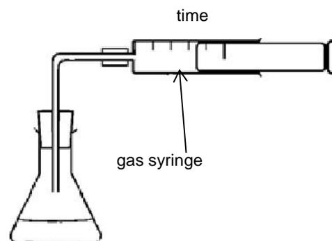
The initial rate is the rate at the start of the reaction, where it is fastest. It can be calculated from the gradient of a continuous monitoring conc vs time graph at time = zero. A measure of initial rate is preferable as we know the concentrations at the start of the reaction.
