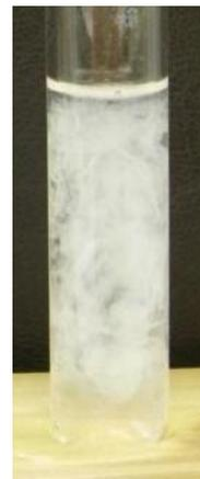
The hydrochloric acid is needed to react with carbonate impurities that are often found in salts which would form a white Barium carbonate precipitate and so give a false result. You could not use sulphuric acid because it contains sulphate ions and so would give a false positive result.
