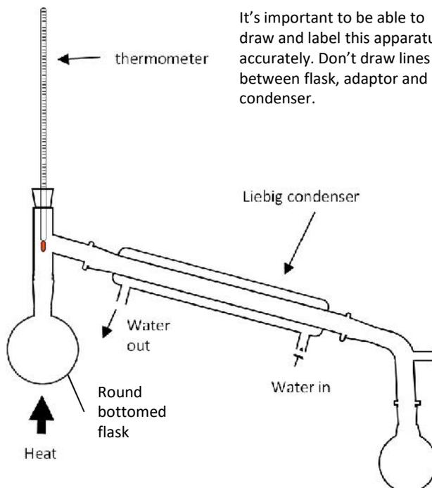
It's important to be able to draw and label this apparatus accurately. Don't draw lines between flask, adaptor and condenser.
