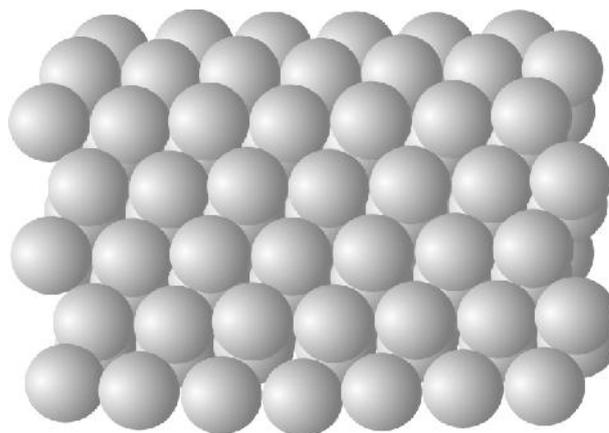
Metals are malleable because the positive ions in the lattice are all identical. So the planes of ions can slide easily over one another. The attractive forces in the lattice are the same whichever ions are adjacent
