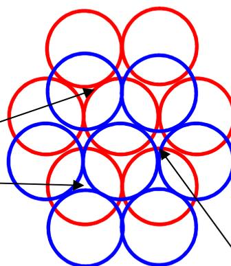
An octahedral site exists when 3 atoms from one each of two layers in the lattice touch each other.
