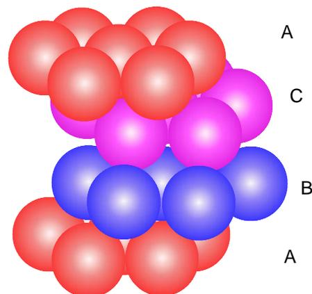
This is the unit-cell representation for cubic close packing. This packing is also called face-centred cubic packing. You can see there are particles at the centre of each face of the unit cell.
