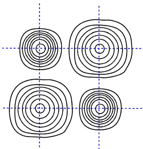
The ions are discrete or separate, because the electron density falls to zero between the ions
