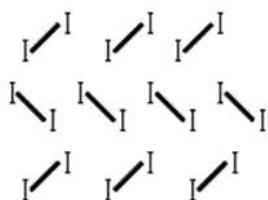
The crystals contain a regular arrangement of I<sub>2</sub> molecules held together by weak van der Waals intermolecular forces
