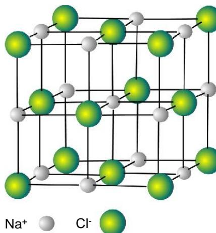
Ionic bonding is between ions and all their surrounding oppositely charged ions. Each sodium ion in this structure is surrounded and equally attracted by six chloride ions. The ionic bond is the attraction between all these ions
