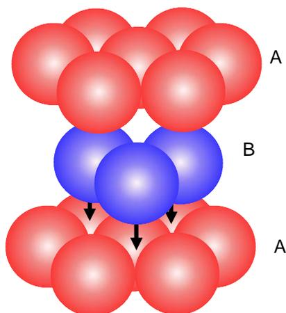
In hexagonal close packing the metal ions are arranged in layers. The second layer (B) sits in the holes above the first layer(A). The pattern continues ABABAB
