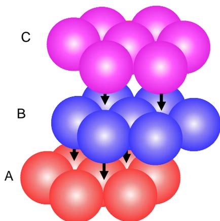
In Cubic Close Packing the layers are arranged differently from hexagonal close packing. The second layer (B) sits in the holes above the first layer (A) in the same way but the third layer does not sit above the first. The third layer is displaced over and is called layer (C).
