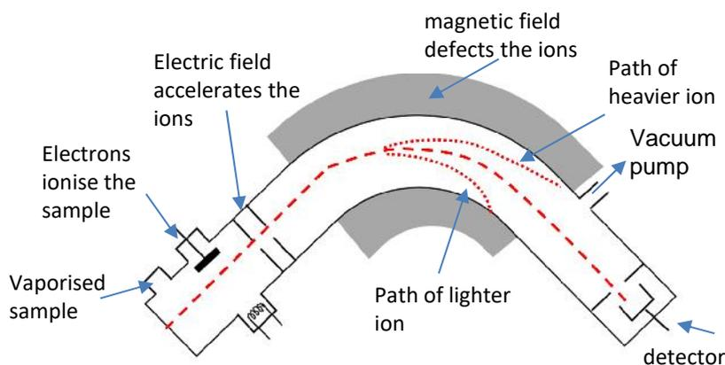
The mass spectrometer can be used to determine all the isotopes present in a sample of an element and to therefore identify elements.
