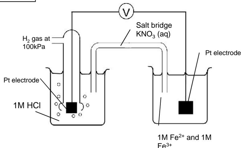
Note: in the electrode system containing two solutions it is necessary to use a platinum electrode and **both** solutions must be of a 1M concentration.
