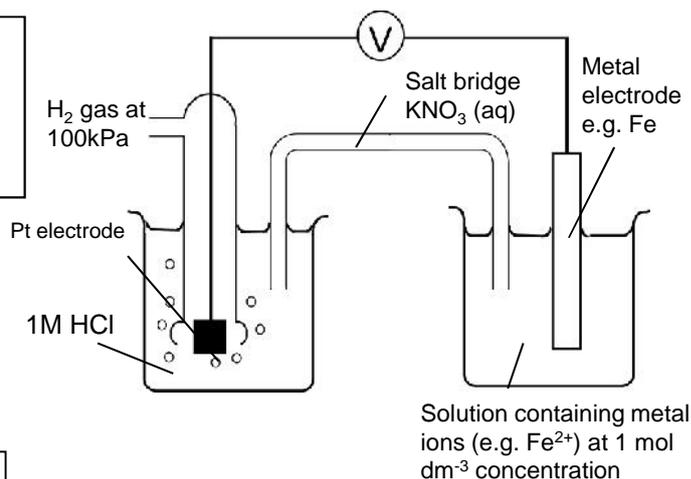
Because the equilibrium does not include a conducting metal surface a platinum wire is used which is coated in finely divided platinum. (The platinum black is used because it is porous and can absorb the hydrogen gas.)
