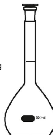
Remember to fill so the bottom of the meniscus sits on the line on the neck of the flask. With dark liquids like potassium manganate it can be difficult to see the meniscus.
