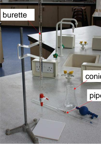
The photograph shows a laboratory setup for titration. A burette is mounted on a stand. A conical flask is placed on the bench next to a pipette and a blue bulb. Labels with red arrows point to the burette, conical flask, and pipette.
