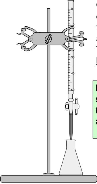
One substance (generally the one we don't know the concentration) is put in the conical flask. It is measured using a volumetric pipette. The other substance is placed in the burette
